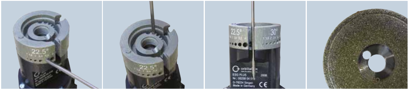
Grinding electrodes: – 4 different angles, 6 different electrode diameters
