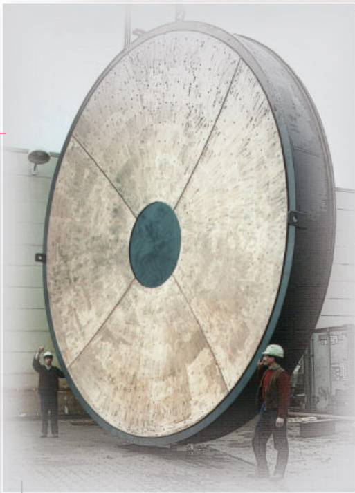
FURNACE FLOOR NAMAKWA SANDS \varnothing 7.0 M
