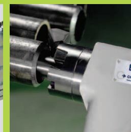
Precise and reproducible pipe end and tube sheet joint preparations.
